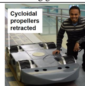
Fig 13. Amphibious UUV in ground mode (cyclo-props stowed).
